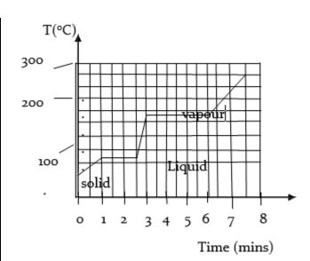
31. If the gas is cooled at what temperature will start to condensate?
